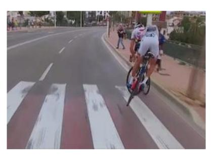
The other big no no is grabbing your front brake whilst cornering. This is most likely to end up with you crashing because the front wheel will tend to wash out. If you have to brake, try to straighten your bike first and then apply your brakes gently. Once in control again, you can apply the brakes progressively harder.
